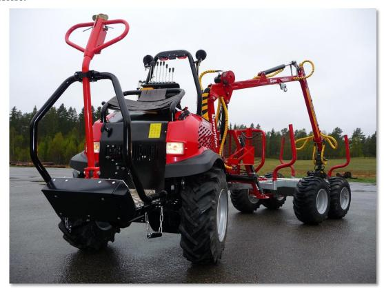
We have used well-tried technology solutions from Iron Horse and combined this with the need for a new "thinning forwader" to the small-scale forestry. Just as the Iron Horse The Wheel Horse is a complete system for forest, farm and transport in different terrain. Flexibility, strength, and low ground pressure makes it an environmentally friendly alternative to heavier machines. The machine is easy to operate and easy to get started and work with.
