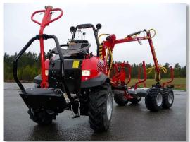
The WheelHorse is equipped with the reliable Honda engine of 13 Hp The vehicle is unique with its mechanical transmission and high- and low gear. The hydraulic engagement on the trailer is easy to control from the steering handle and the machine has 6 wheel traction, when there are need extra power for pulling. The trailer is equipped with a powerful grip that have a big lift capacity comparing to it size.
